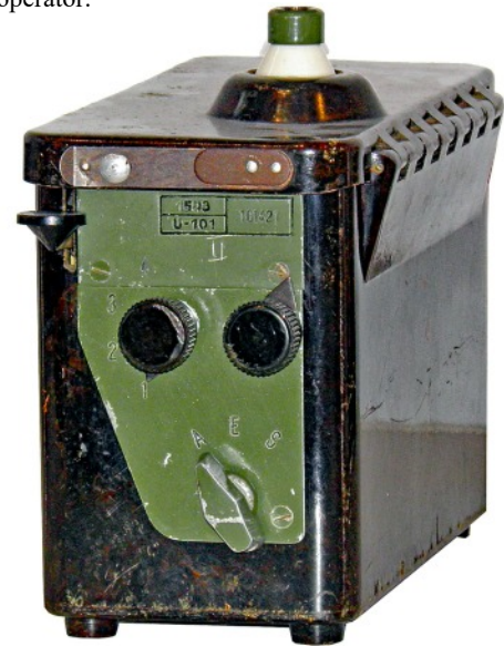
Right hand side panel with control panel and a panel with type, serial number and (believed to be) the code number of the maker.
